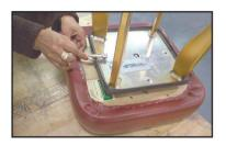
Place chair on bench up side down. Using two 7/16" wrenchs, remove the four bolts holding the base on. Remove the base and set right-side up away from the work area.
