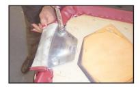
With one hand hold the back plate. Use a 1/2" wrench to remove the two remaining bolts on the back plate. Set aside the back.
