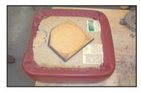
Staple the new seat sewing on. As you work your way around the seat, pull the covering tight and make sure the fabric is laying smooth on the side of the cushion.
