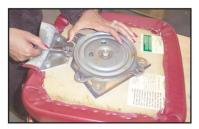
With one hand rotate the swivel mechanism until the bolts holding it on the seat, are visible. With the other hand, use a 7/16" wrench to remove these four bolts. Remove swivel mechanism.
