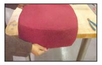
Pull the seat cover down over the cushion working your way around the cushion. Make sure the seam is centered on the back of the seat. Pull down snug. Carefully position the top seam as pictured above.
